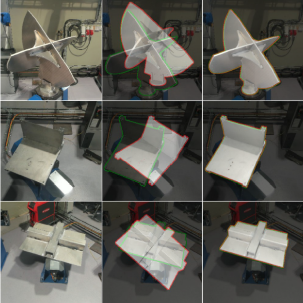
Figure 11: Test set examples with CosyPose. The image from the camera is shown to the left, the initial pose estimate in the middle, and the final pose estimate after five prediction iterations to the right.
